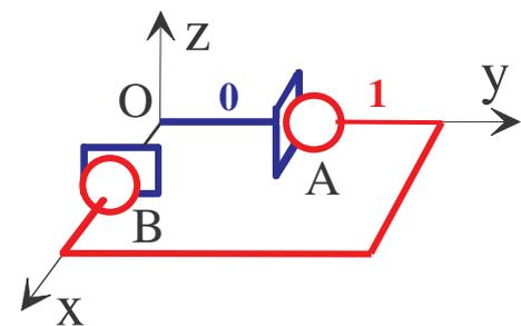
$$\left\{ V_{1/0}^{L_A} \right\} = \begin{Bmatrix} \alpha_A & u_A \\ \beta_A & 0 \\ \gamma_A & w_A \end{Bmatrix}_{A, B_0} \quad \left\{ V_{1/0}^{L_B} \right\} = \begin{Bmatrix} \alpha_B & 0 \\ \beta_B & v_B \\ \gamma_B & w_B \end{Bmatrix}_{B, B_0}$$
