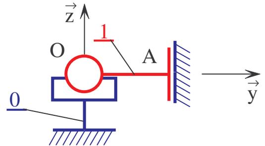
$$\{V_{1/0}^{L_A}\} = \begin{Bmatrix} 0 & u_A \\ \beta_A & 0 \\ 0 & w_A \end{Bmatrix}_{A,B_0} \quad \{V_{1/0}^{L_O}\} = \begin{Bmatrix} \alpha_O & 0 \\ \beta_O & v_O \\ \gamma_O & 0 \end{Bmatrix}_{O,B_0}$$
