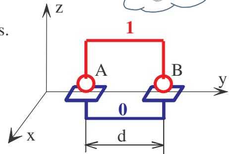
$$\left\{ V_{1/0}^{L_A} \right\} = \begin{Bmatrix} \alpha_A & u_A \\ \beta_A & v_A \\ \gamma_A & 0 \end{Bmatrix}_{A, B_0} \quad \left\{ V_{1/0}^{L_B} \right\} = \begin{Bmatrix} \alpha_B & u_B \\ \beta_B & v_B \\ \gamma_B & 0 \end{Bmatrix}_{B, B_0}$$
