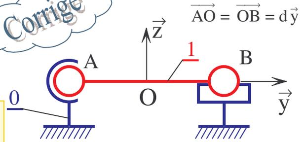
$$\{V_{1/0}^{L_A}\} = \begin{Bmatrix} \alpha_A & 0 \\ \beta_A & 0 \\ \gamma_A & 0 \end{Bmatrix}_{A,B_0} \quad \{V_{1/0}^{L_B}\} = \begin{Bmatrix} \alpha_B & 0 \\ \beta_B & v_B \\ \gamma_B & 0 \end{Bmatrix}_{B,B_0}$$
