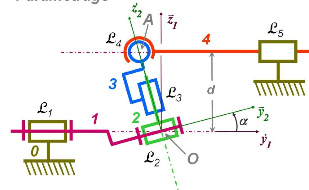
$$\left\{ \mathcal{V}_{1/0} \right\} = \begin{matrix} \text{O} \\ \beta_1 \cdot \vec{y}_1 \\ \vec{0} \end{matrix} \quad \left\{ \mathcal{V}_{2/1} \right\} = \begin{matrix} \text{O} \\ \beta_2 \cdot \vec{y}_2 \\ \vec{0} \end{matrix} \quad \left\{ \mathcal{V}_{3/2} \right\} = \begin{matrix} \text{O} \\ \gamma_3 \cdot \vec{z}_2 \\ \omega_3 \cdot \vec{z}_2 \end{matrix}$$
